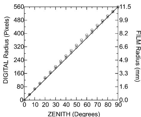
Fig. 3. Radial calibration data measured for the Nikkor 8 mm  $f/8$  fisheye lens (+), the Nikon Coolpix 950 and FC-E8 fisheye converter ( $\times$ ), and the well-documented Nikkor 8 mm  $f/2.8$  (○), which replaced the older Nikkor 8 mm  $f/8$  lens c. 1970. The straight line represents a perfect polar (equiangular) projection.
