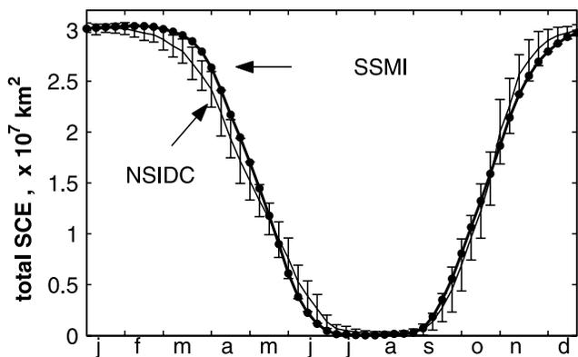
**Figure 1.** Seasonal variation of the total snow cover extent (total SCE) over Canada-Alaska and northern Eurasia derived from the thresholded microwave brightness temperature approach (SSM/I: dot and bold line) and from the Northern Hemisphere EASE-Grid Weekly Snow Cover and Sea Ice Extent NSIDC product (shaded line, with error bars) for the 1988–2001 period. Error bar data correspond to 1 standard deviation.
